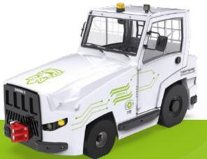
»SHERPA« E Max towed load ≤ 60 t 40 kW | 1x 35 kWh battery 35 kN Drawbar pull »SHERPA« E Max towed load ≤ 80 t\* 70 kW | 2x 35 kWh batteries 45 kN Drawbar pull
