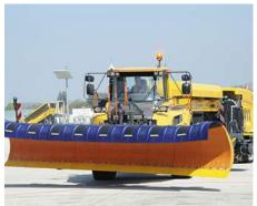
The broom length is 5,600 mm. The broom length is 6,300 mm.
