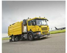
The AS 990 series machine can also be equipped as a stand cleaning machine. The stand cleaning option is particularly suitable for collecting rubber abrasion and oil.
