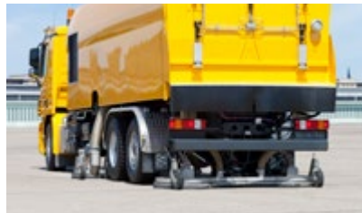
Truck with lowered rear cleaning device (working position) (3 x 850 mm Ø) and one lowered demarking device (left side).
