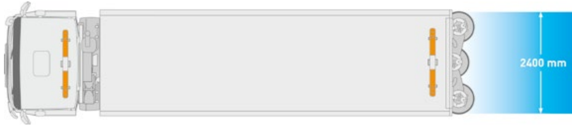
Truck with lowered rear cleaning device (working position) (3 x 850 mm Ø) and one lowered demarking device (left side).
