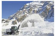
The high-capacity Supra 5002 can be equipped with hydraulically movable front flaps especially for use at airports. This increases the clearing width and can be flexibly adapted to the width of the snow bank, allowing particularly efficient snow removal. In addition to its great clearing efficiency, the Supra's all wheel drive makes it highly manoeuvrable – very important in narrow areas on airports and near aircraft.
