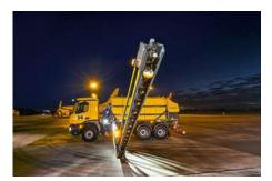
The solid parallelogram construction at the front of the machine ensures safe quidance of the spraying arms. The outer spraying arm sections are made of aluminium and have collision protection through a break-out system.
